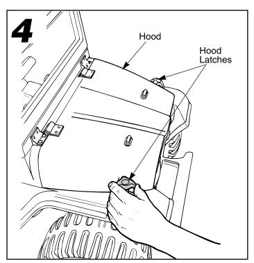
Lower the hood. Lift the hood latches and fit the short tabs onto the notches on the hood to fasten it.
